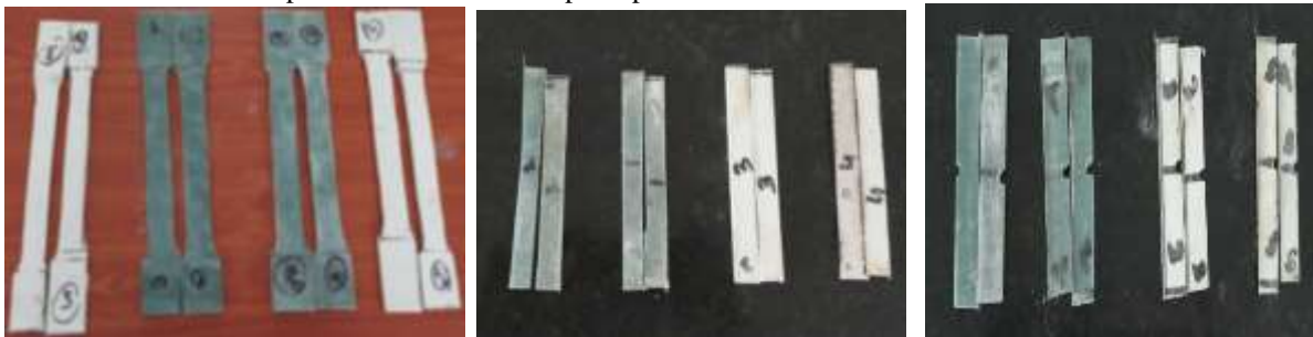
Fig: 3: Tensile, flexural and Impact test Specimens
